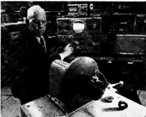
Balderston listens in on bearing failure. Wired for sound, bearing sings worried song.
