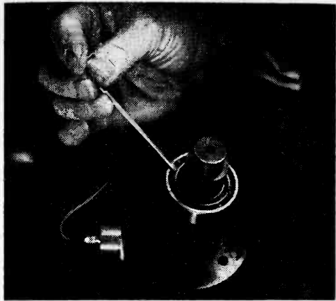
Adding oil to ball bearing just might improve operation; sounds tell for sure.
