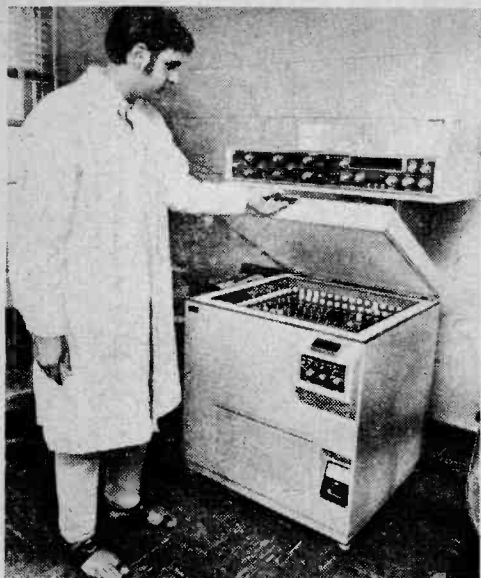
One way to check marine growth is to use radioactive "tags" in the food cycle. Then, electronic circuits measure isotope emissions.
